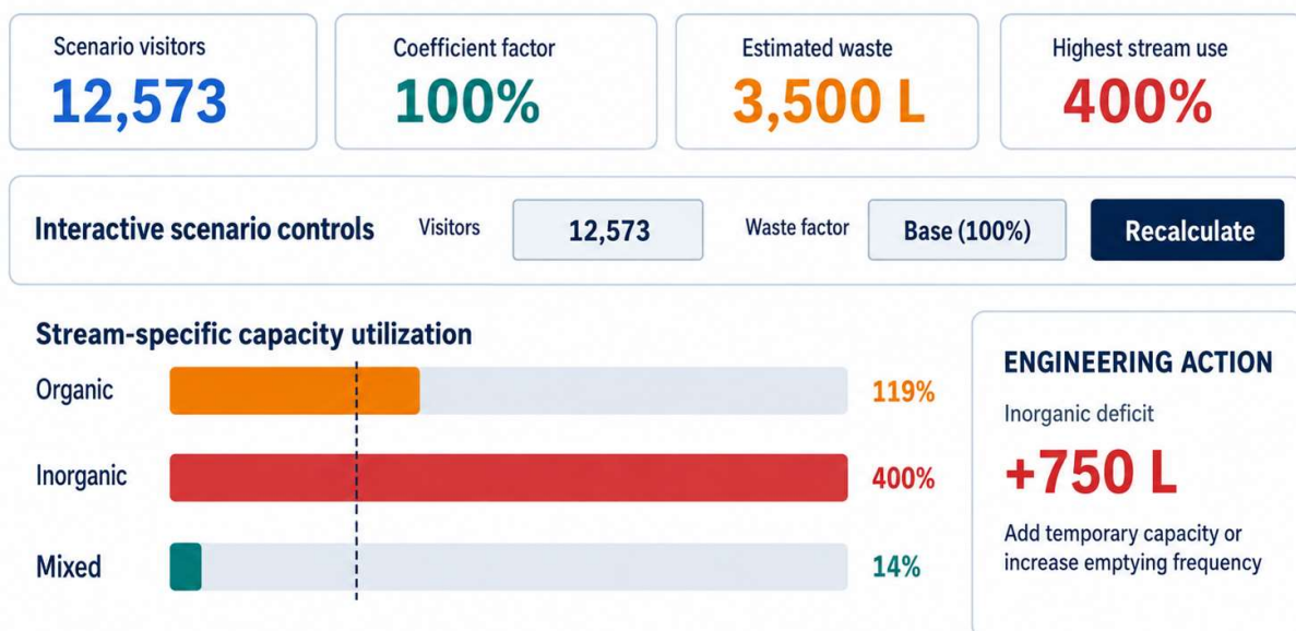
Figure 5. Interactive scenario-assessment prototype with stream-level capacity rules and an interpretation safeguard.
