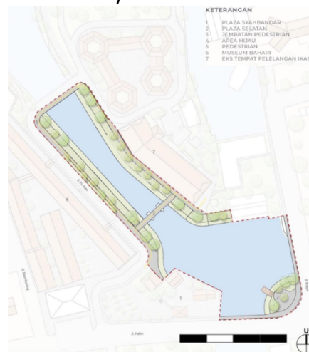
Figure 18. Bahari Diversion Channel – Conceptual Site Plan of the East Canal
