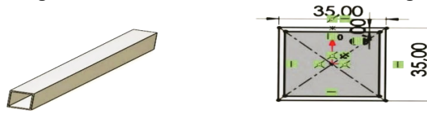
Figure 2. Hollow profile used as the frame material
