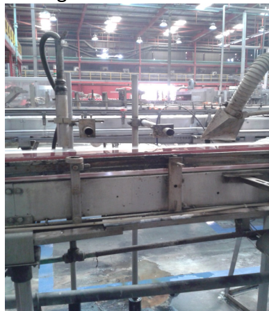
Figure 7. Automated Date Coding Process
