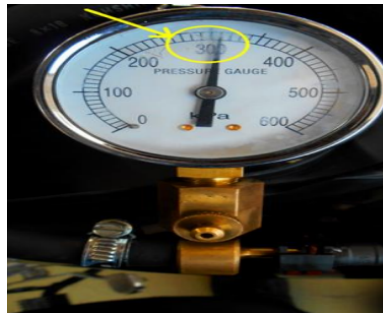
Figure 14. Fuel Injection Pump Pressure Measurement
