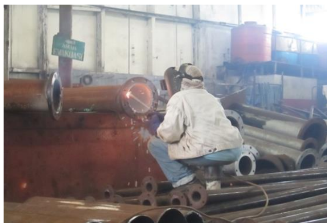
Figure 3. Upper Hand Welding Technique at a 45° Hand Position
