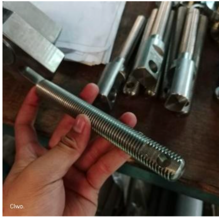
Figure 6. Result of Making Lifter Guide Shaft
